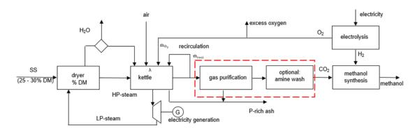
A simulation software (Aspen Plus) is used to model a combination of a power plant and a P2X process. The methanol production using carbon dioxide and hydrogen is analyzed as an exemplary P2X process. The oxygen for the O2-enriched combustion and the hydrogen for the chemical synthesis come from water electrolysis.
