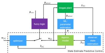
However, the model based control system needs a detailed mathematical model of a biogas plant to be able to produce an efficient control method. Use of a diverse type of feeding in addition to constantly changing chemical and biological parameters in the fermenter add the complexity to create model analytically. Therefore, machine learning approach is used.
