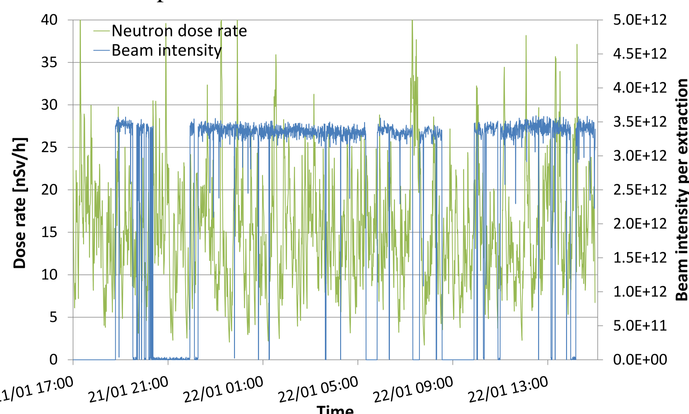
Figure 6. SPS beam intensity vs neutron H*(10) for the position 1.
