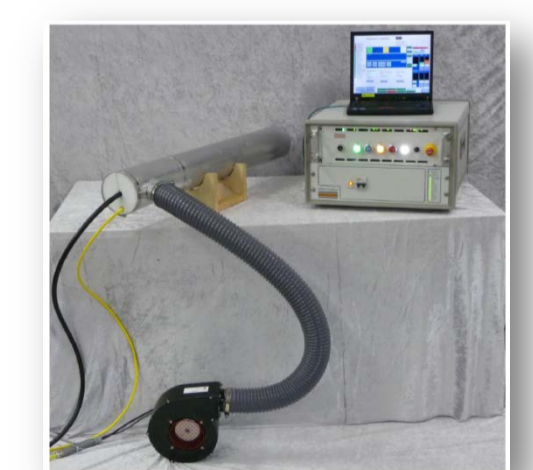
Figure 17. NSD-35 Neutron Generator by Gradel s.a.r.l.
