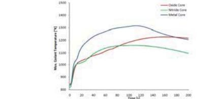
Fig. 13: Peak coolant T. during loss of IHTS cooling with station blackout
