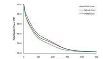
Fig. 11: Reactor power during loss of IHTS cooling with station blackout
