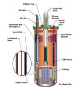
Fig. 5: S-PRISM Reactor core
