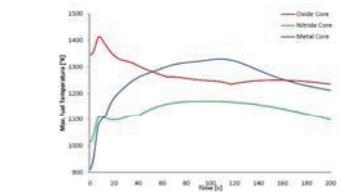
Fig. 12: Peak fuel temperatures during loss of IHTS cooling with station blackout
