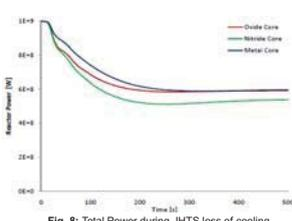
Fig. 8: Total Power during IHTS loss of cooling
