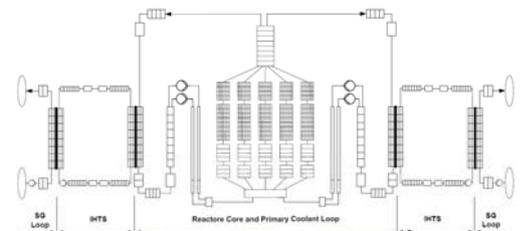
Fig. 6: RELAP5 S-PRISM nodalization
