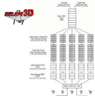
Fig. 2: S-PRISM core nodalization
