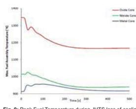
Fig. 9: Peak Fuel Temperature during IHTS loss of cooling
