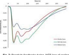
Fig. 7: Reactivity feedbacks during IHTS loss of cooling
