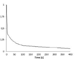
Fig. 10: Primary flow coastdown during loss of power
