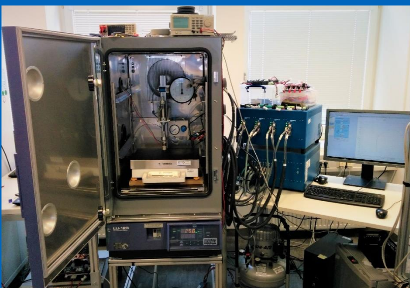
Electrochemical Impedance Spectroscopy (EIS) measurements being carried out within a temperature-controlled environment.
