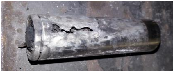
Fresh commercial cylindrical lithium-ion battery (at the top) and a battery after a thermal runaway showing side rupture (at the bottom).
