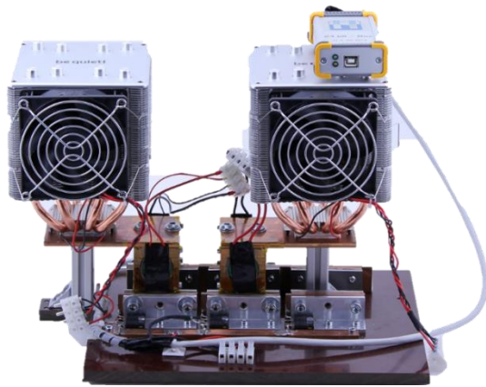
Testbench to measure the current distribution within two parallel connected cells with optional individually controlled temperature of each cell.
