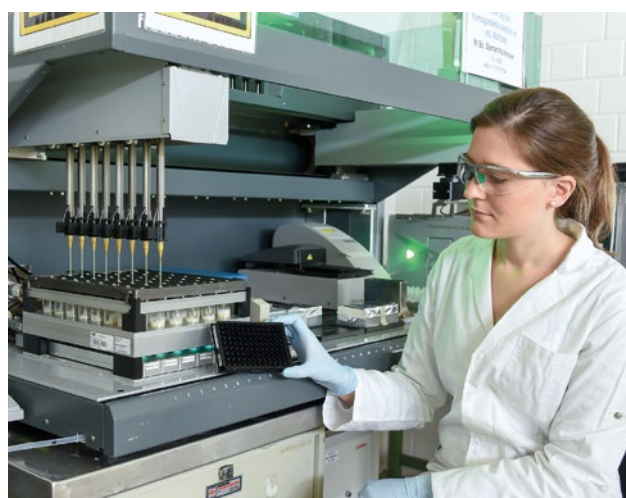
Operation of a bioreactor unit with 48 parallel single-use stirred-tank bioreactors on a milliliter-scale (photo: Tobias Hase, TUM)
