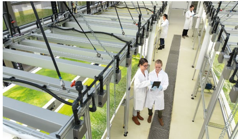
New open thin-layer cascade photobioreactors operated in the TUM Algae TechCenter, Ottobrunn (photo: Tobias Hase, TUM)
