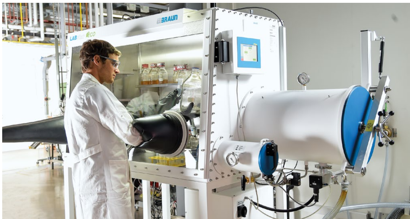
Special microorganisms are able to produce chemicals with carbon dioxide as sole carbon source, but oxygen (air) is toxic to them. At the Institute of Biochemical Engineering these microorganisms are prepared in anaerobic (oxygen free) workbenches for reaction engineering studies in bioreactors. (photo: Tobias Hase, TUM)
