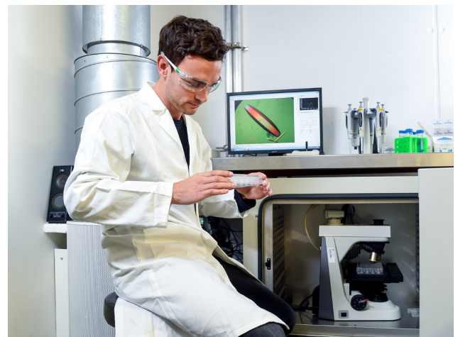
Protein crystallization is studied in parallel in a temperature-controlled incubator. Crystal formation is monitored automatically with a microscope (photo: Tobias Hase, TUM)
