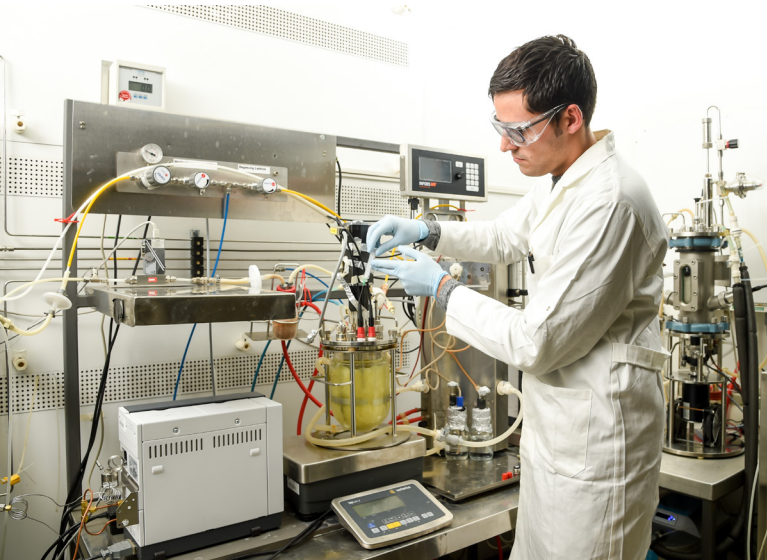
Special syngas-converting microorganisms are studied in fully controlled stirred-tank bioreactors operated in a syngas ( \text{CO}_2 , \text{H}_2 , CO) compartment of the lab ensuring safety requirements are met. (photo: Tobias Hase, TUM)
