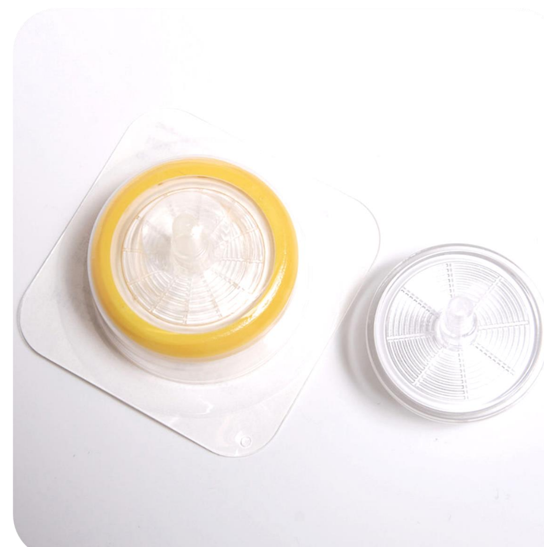
0.22 \mu\text{m} syringe filter Those filters are typically used for sterile filtration, but are not useable for our use case.
