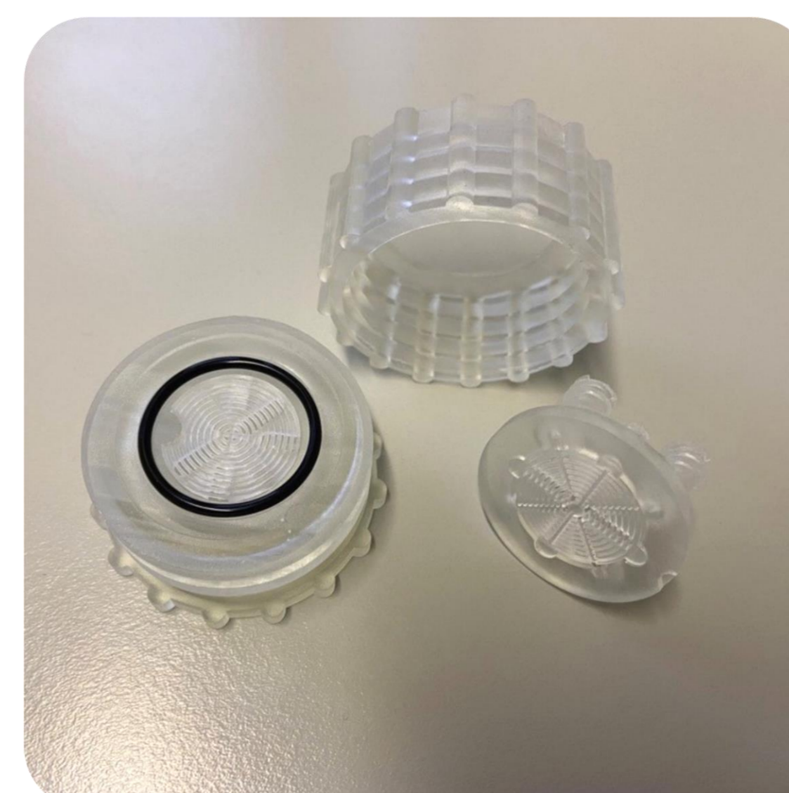
3D printed Membrane holder Current iteration of the membrane holder. Printed on a FormLabs 3B SLA printer.
